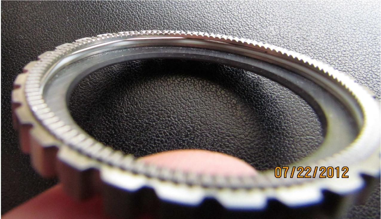
Make sure the bezel click spring is properly installed on the case. There is a "foot" on the spring that will fit into a hole in the case.
