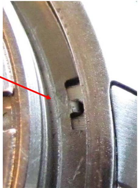
Place the ceramic bezel on the case and push down. You will hear it "snap" on. Check to make sure it properly rotates.
