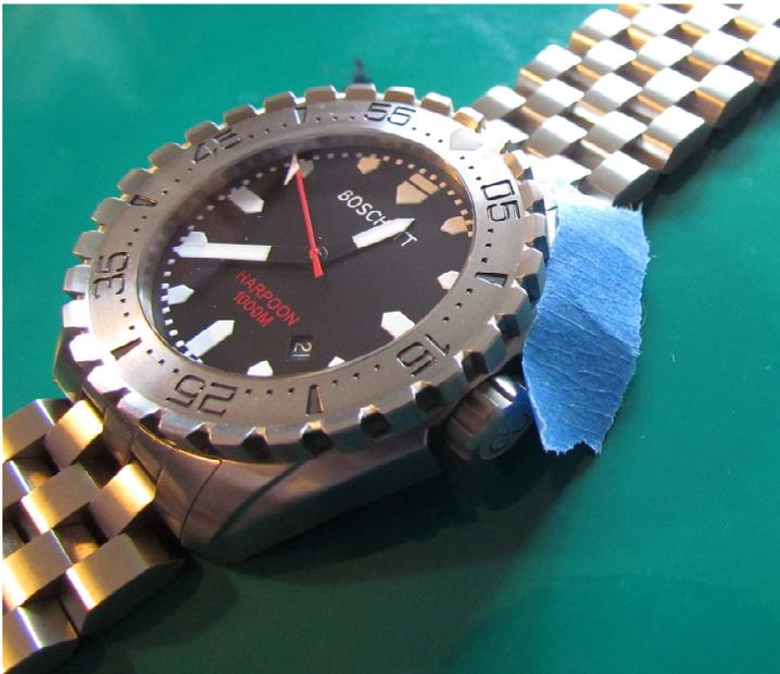
Slide the blade between the case and bezel. The bezel should "pop" off. Twisting or pushing up on the blade may be necessary.
