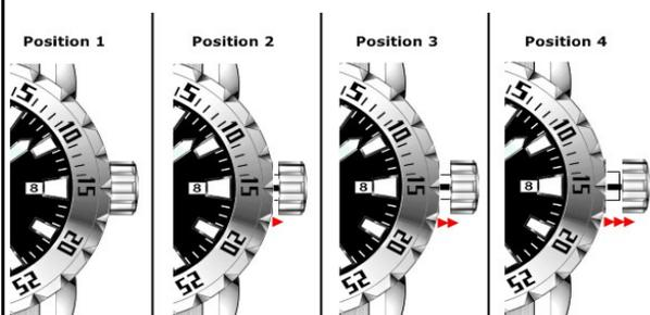
**Important information:** Your watch has a self-winding movement and a screw down crown. To maintain proper working order, the crown must be screwed down to position 1 during normal wear. The watch is also water resistant. In order to be in compliance with the warranty, the crown must also be screwed down while exposing the watch to water.
